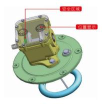
Adopt incomplete bevel gear transmission technology of operating mechanism. The output angle is accurate to ensure the reliable operation of the tap changer; the input angle tolerance range is wide, and the input safety position area display is set, which is convenient for installation, connection and operation with high reliability.
